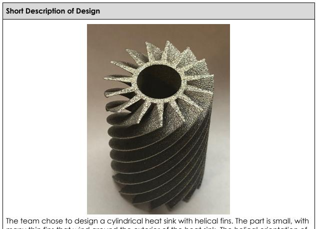
The team chose to design a cylindrical heat sink with helical fins. The part is small, with many thin fins that wind around the exterior of the heat sink. The helical orientation of the fins increases the surface area of the part, without increasing the overall volume as compared to a similarly designed part with straight fins. This would likely increase the heat transfer without taking up more space in an assembly.
