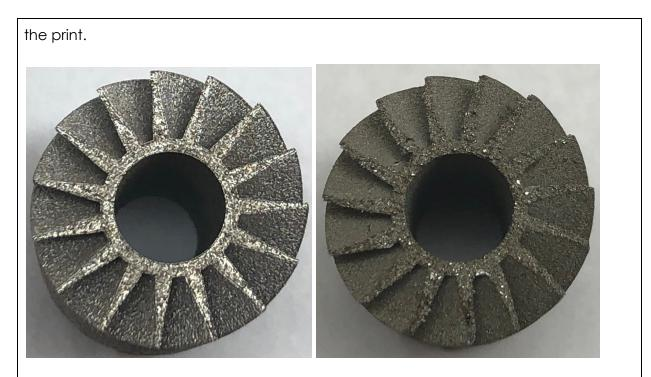
Shown above: The top face of the spiral heat sink (left), and the bottom face (right) where supports were removed.
