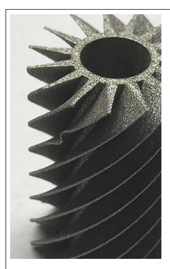
Above: A small wrinkle is present on one fin near the top of the part.
